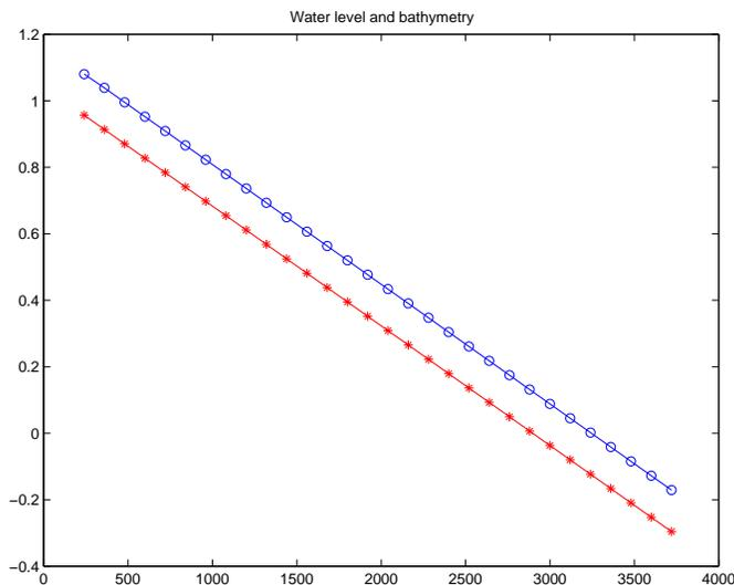
Figure 4: *Computed water levels (blue) and bottom depths (red, shifted upwards by 5.5 m) along the center line of the river section in test model 1, using a straight grid.*
