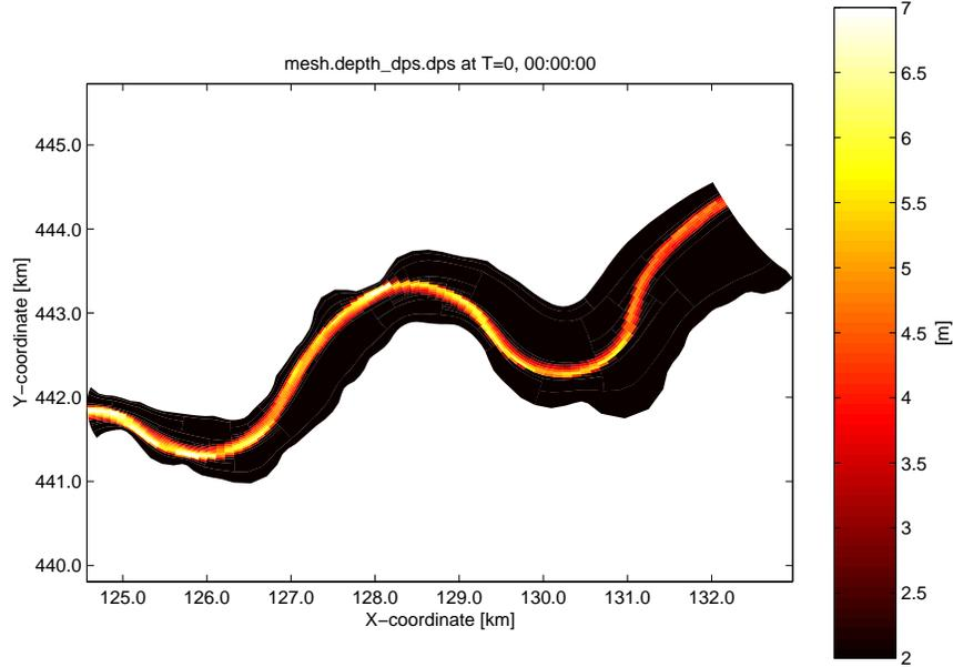
Figure 1: *Bottom depth in a river section (Lek) of the Zeedelta model.*
