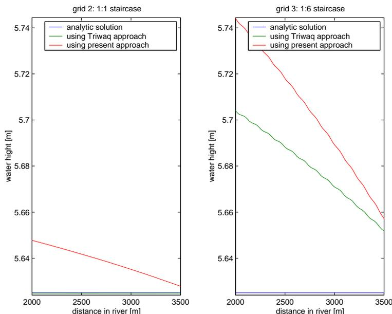
Figure 7: Water depths along the centerline of the river section for the rotated grids for a situation with horizontal viscosity,  $\nu_h = 6\text{m}^2/\text{s}$ . Left: grid 2, full staircase boundary, right: grid 3, sideways step at every sixth forward step.
