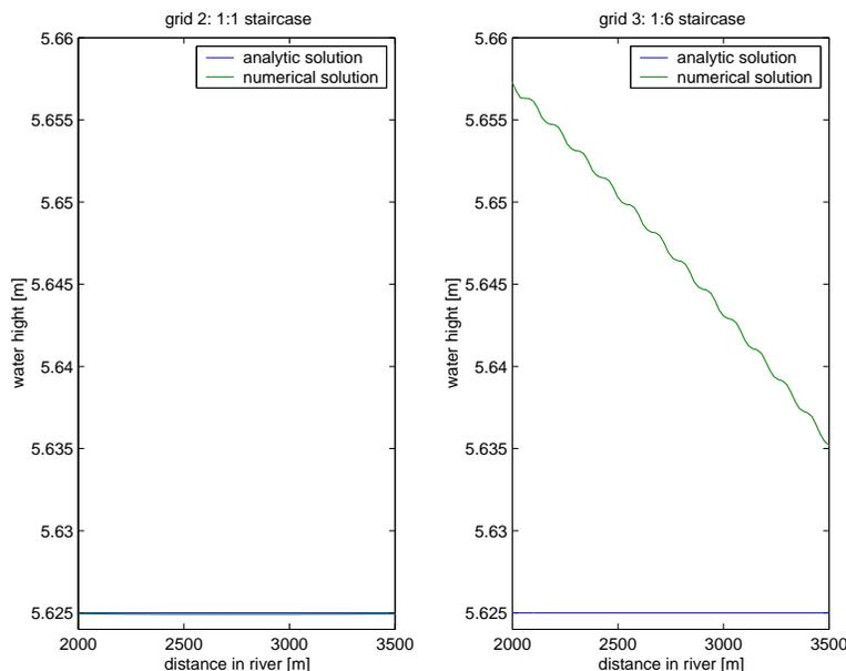
Figure 5: Water depths along the centerline of the river section for the rotated grids for a situation without horizontal viscosity,  $\nu_h = 0$ . Left: grid 2, full staircase boundary, right: grid 3, sideways step at every sixth forward step.
